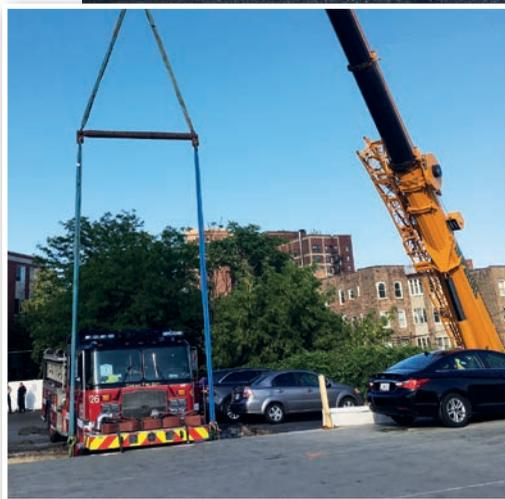
**The front bumper was the only thing holding the fire truck in place. (Inset) With the firetruck having no lifting point, Imperial used a 20-ton capacity lifting beam rigged to the bumper.**
