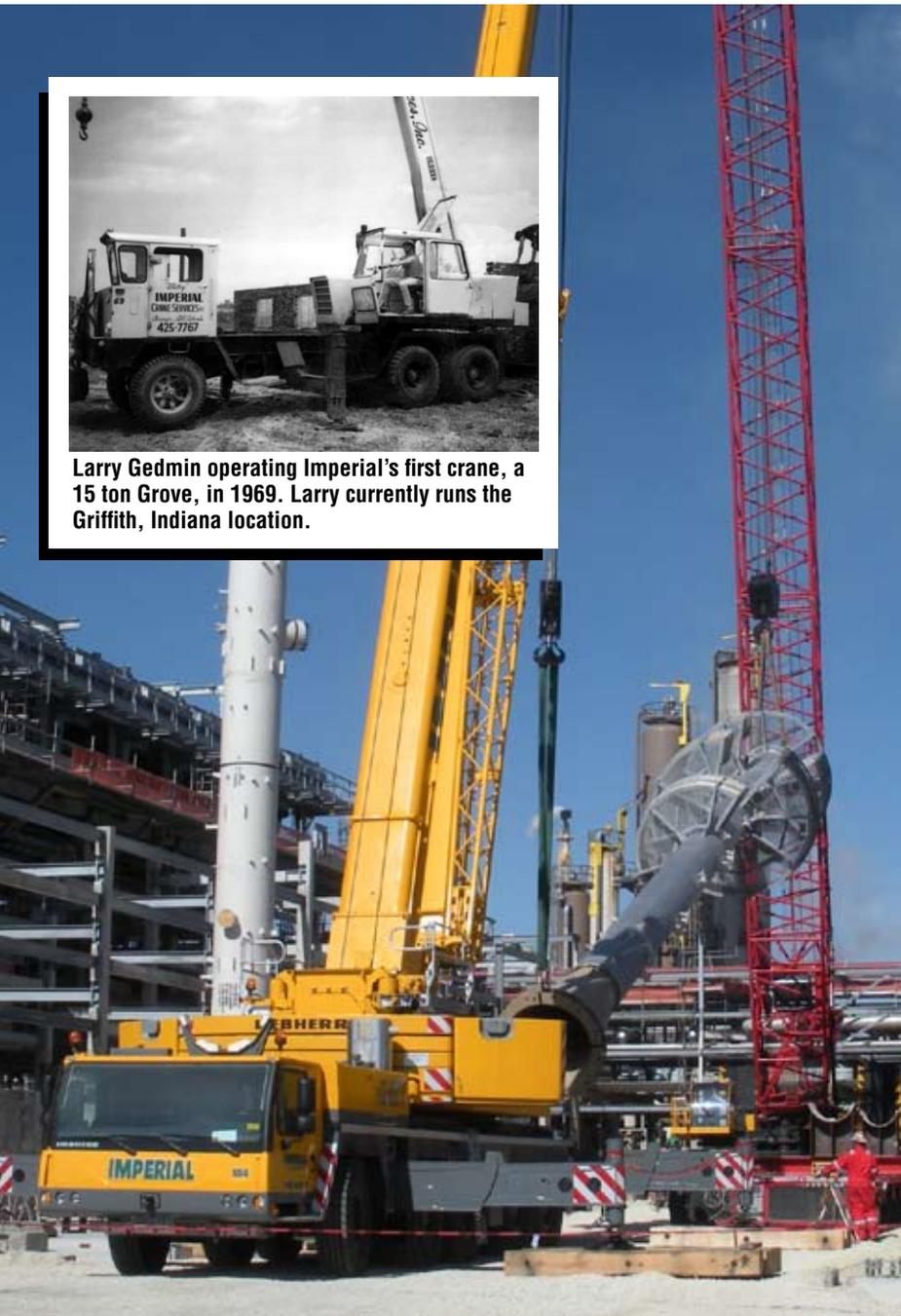
235 ton Liebherr works in tandem with 350 ton Sany crawler at CITGO refinery project.
